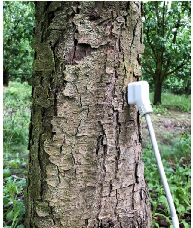
*Figure 1. A SapLinX Sap Flow Sensor installed on the trunk of a pear tree.*
